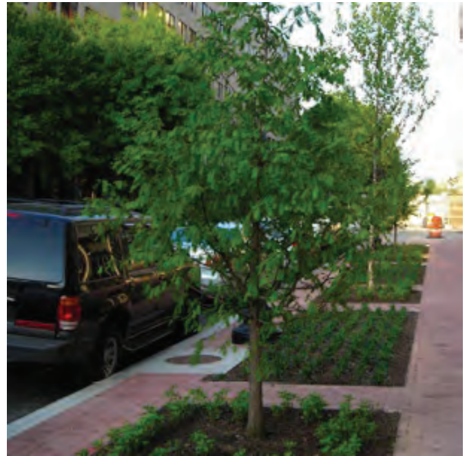
Photo 6-2: Example of a streetscape with adequate soil volume for trees.
